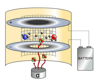
The alpha particles ionize the air creating a current in the smoke alarm. The alarm does not go off.
