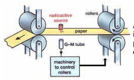
A radioactive source is on one side of the paper and a detector on the other.
